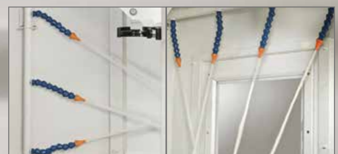
■ Coolant Shower for Efficient Chip Removal < NXV Series std. >
