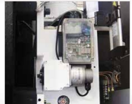
■ Absolute Encoder ATC System < NXV1680B is exclusive >
